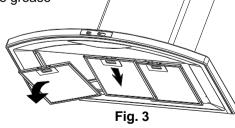
When washing the metal grease filter in the dishwasher a slight discolouration of the filter can occur, this does not have any impact on its performance.
